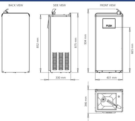
Can be used free standing or wall tight to avoid unsightly connections. Exclusive Projector Design: 2-stream mound-building projector and automatic stream regulator. Plumbing Connections: enter directly into cabinet. Waste 24 mm (1") IPS. Supply 8 mm (3/7") IPS.
