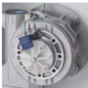
Gear box protection (hall effect)
